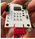
Plug in the USB plug into any open USB port in the machine. You can also use a power brick to plug the USB into to get power. Connect the 5 pin connector to the front of the communication board to the 5 pin plug.
